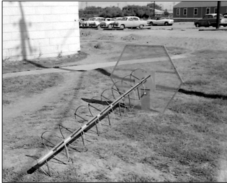
Figure 19. Helical Beam Antenna for Receiving Telemetry Transmissions from Rockets in Flight, 1959
