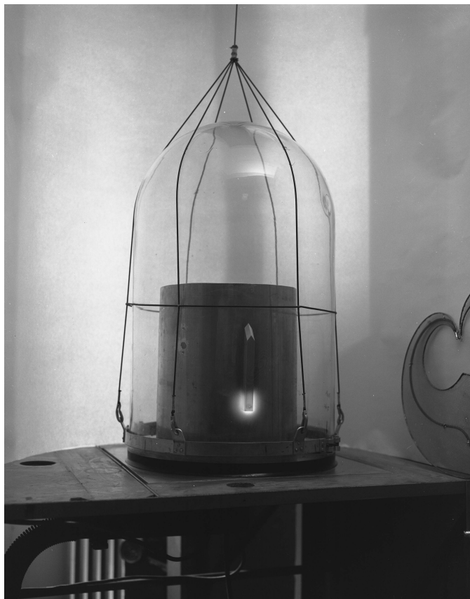
Figure 79. Testing an Antenna in a Bell Jar
