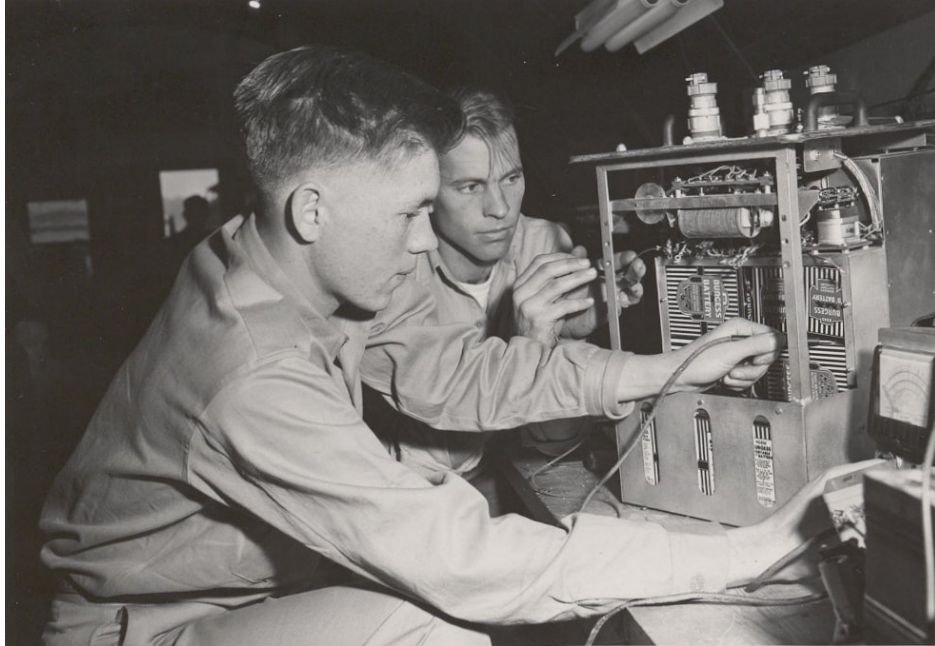
Figure 16. PSL Engineers Robert Sabin and Paul Hill Check Dry-Cell Power Pack to be Flown in a V-2 Rocket, 1947
