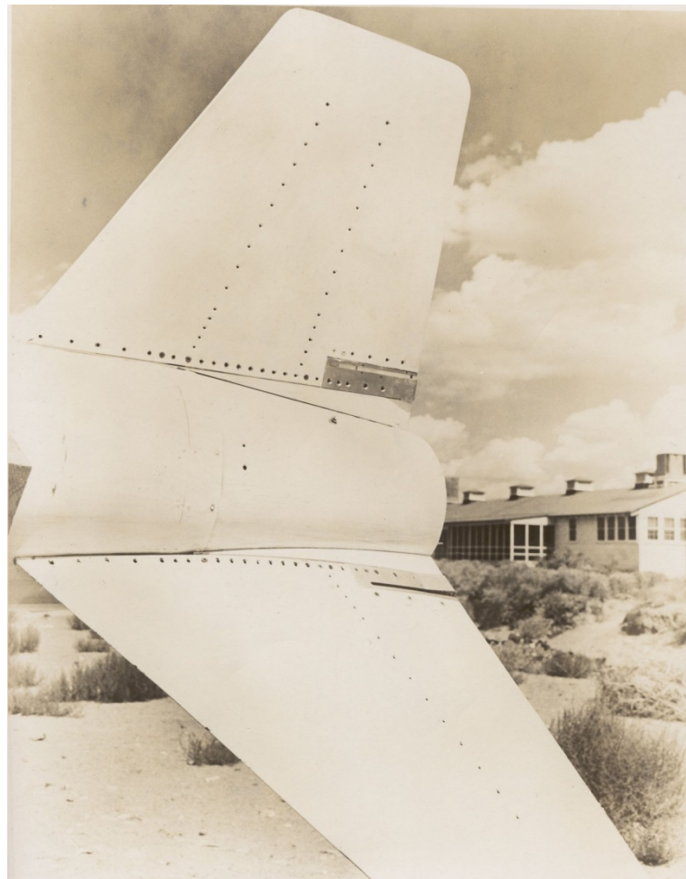
Figure 26. Notch Pair Installed in Fins
